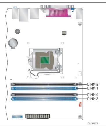
Figure 3. Memory Channel and DIMM Configuration
