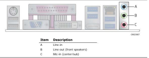
**Figure 4. Back Panel Audio Connectors**
