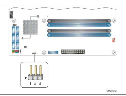
Figure 15. Intel MEBX Reset Header
