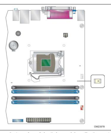
Figure 8. Location of the Enhanced Standby Power LED
