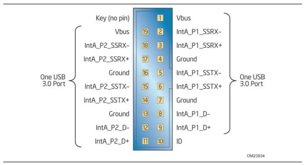
Figure 13. Connection Diagram for the Front Panel USB 3.0 Connector
