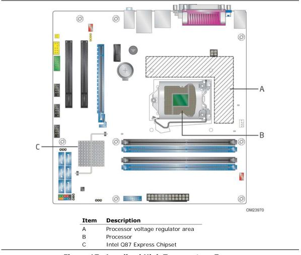
**Figure 17. Localized High Temperature Zones**
