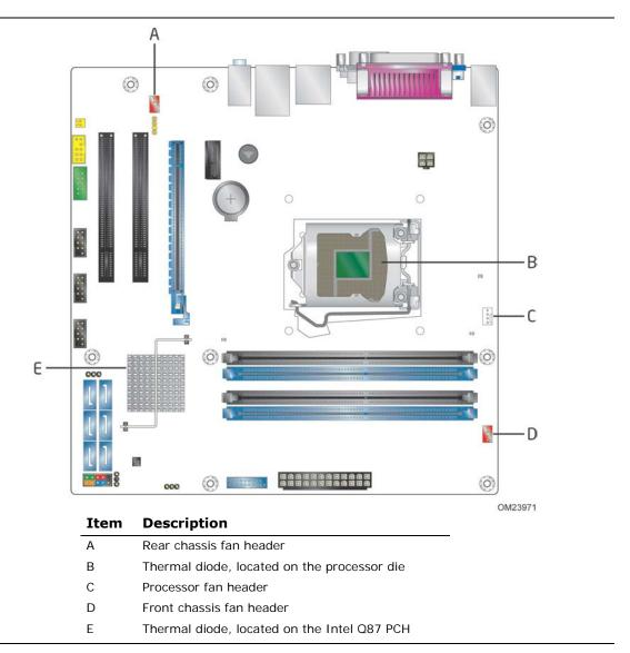
Figure 6. Thermal Sensors and Fan Headers
