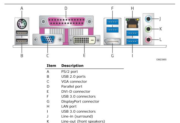
Figure 9. Back Panel Connectors
