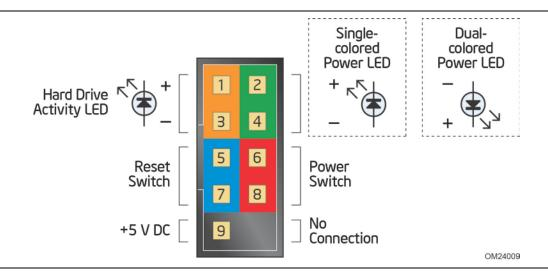
Figure 11. Connection Diagram for Front Panel Connector
