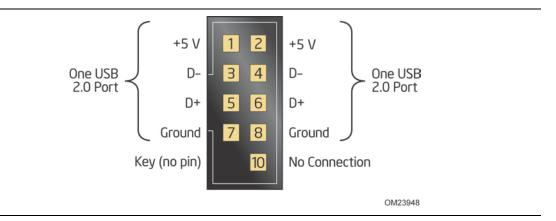
Figure 12. Connection Diagram for Front Panel USB 2.0 Connectors
