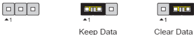
Figure 4 – Clear CMOS jumper
