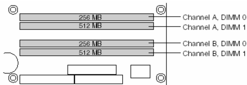
Figure 9. Dual Channel (Interleaved) Mode Configuration with Four DIMMs
