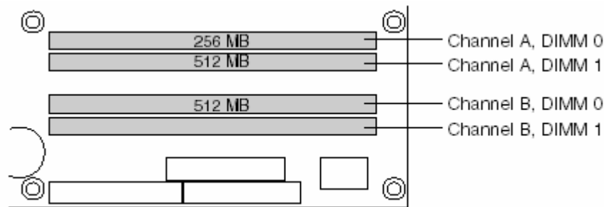
Figure 11. Single Channel (Asymmetric) Mode Configuration with Three DIMMs
