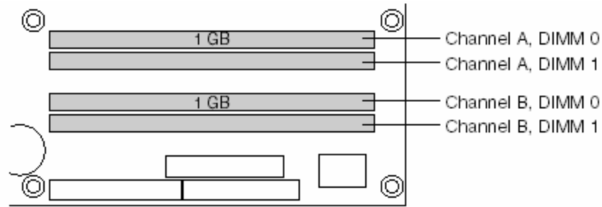
Figure 7. Dual Channel (Interleaved) Mode Configuration with Two DIMMs
