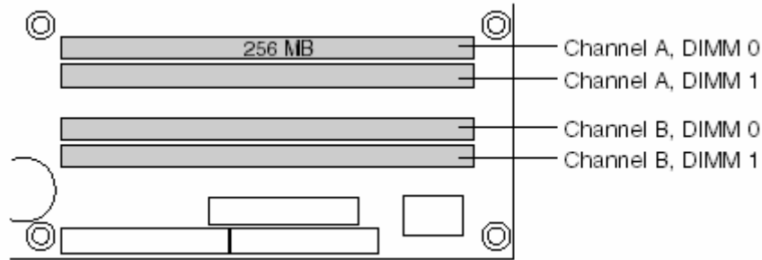
Figure 10. Single Channel (Asymmetric) Mode Configuration with One DIMM
