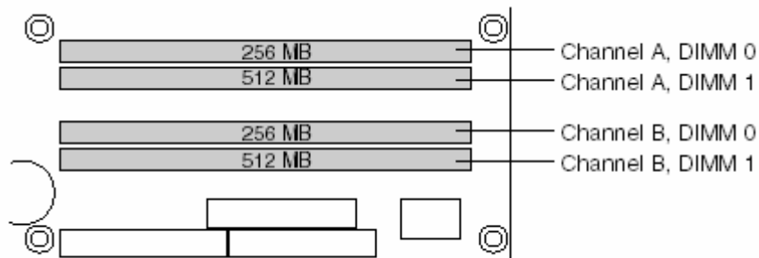
Figure 9. Dual Channel (Interleaved) Mode Configuration with Four DIMMs
