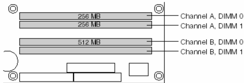
Figure 8. Dual Channel (Interleaved) Mode Configuration with Three DIMMs
