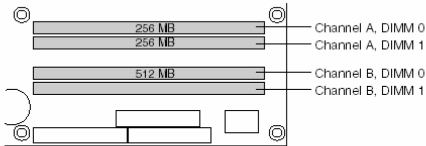
Figure 8. Dual Channel (Interleaved) Mode Configuration with Three DIMMs
