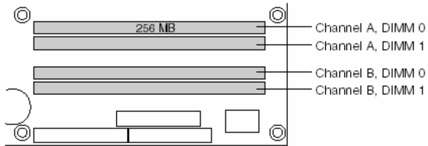
Figure 10. Single Channel (Asymmetric) Mode Configuration with One DIMM
