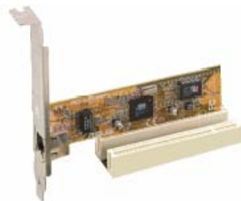
Figure 43: Installing a PCI card
