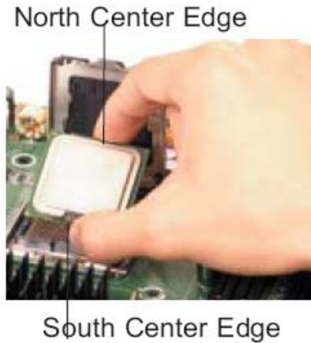
Figure 35: Correct way to hold CPU
