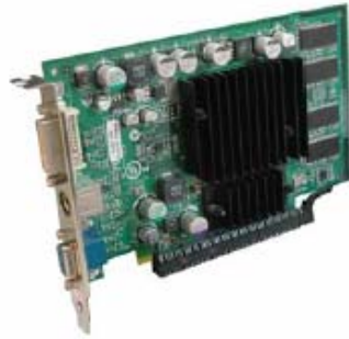
Figure 44: Install a PCI Express x16 card
