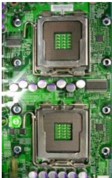
Figure 30: CPU sockets showing Heatsink clips
