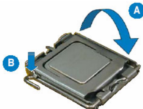
Figure 20: Closing the Load Plate
