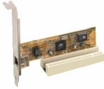
Figure 30: Installing a PCI card
