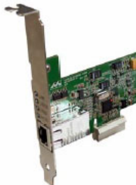
Figure 32: Install a PCI Express x1 card
