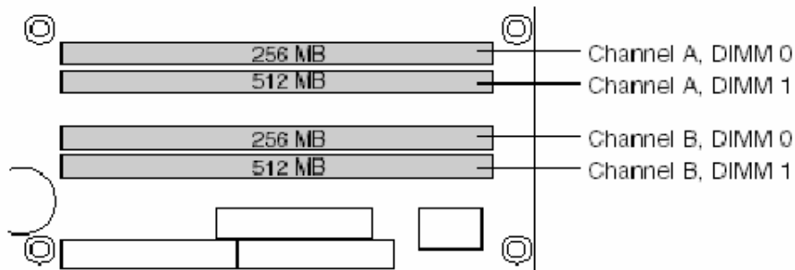
Figure 27: Dual Channel Mode Configuration with Four DIMMs
