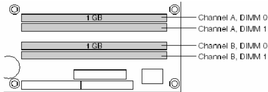
Figure 26: Dual Channel Mode Configuration with Two DIMMs
