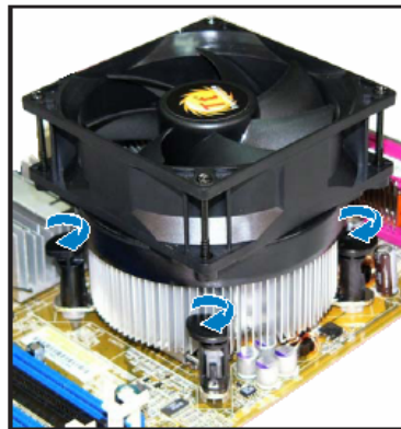
Figure 23: Rotating the Push-Pins
