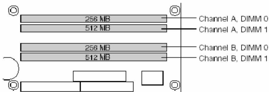
Figure 27: Dual Channel Mode Configuration with Four DIMMs
