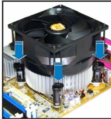
Figure 22: Securing the Heatsink
