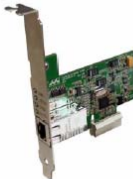
Figure 32: Install a PCI Express x1 card
