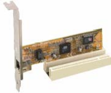
Figure 16: Installing a PCI card
