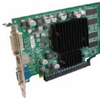
Figure 17: Install a PCI Express x16 card
