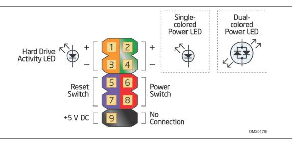
Figure 12. Connection Diagram for Front Panel Header
