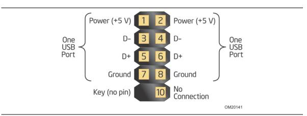
Figure 13. Connection Diagram for Front Panel USB Header
