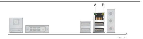
Figure 4. LAN Connector LED Locations
