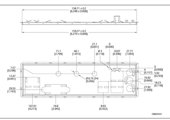
Figure 10. I/O Shield Reference Diagram
