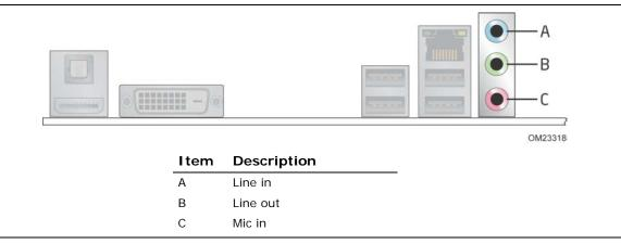
Figure 5. Back Panel Audio Connectors
