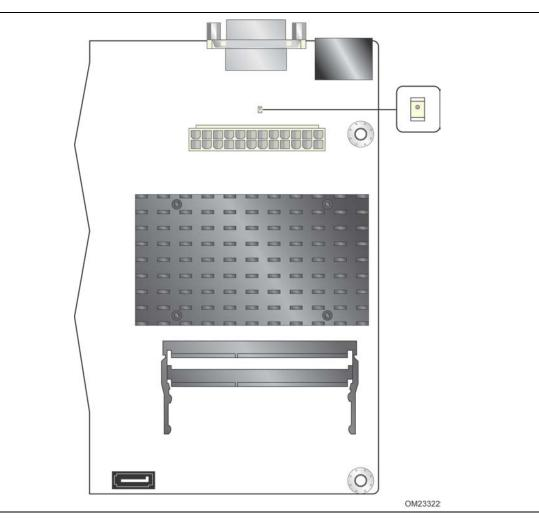
Figure 7. Location of the Standby Power Indicator LED
