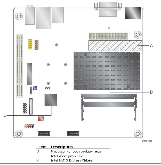
Figure 17. Localized High Temperature Zones
