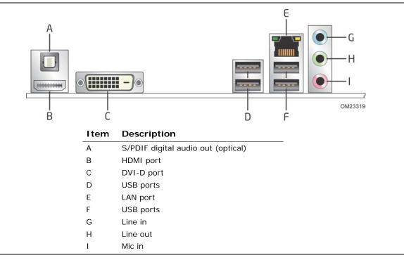
Figure 9. Back Panel Connectors
