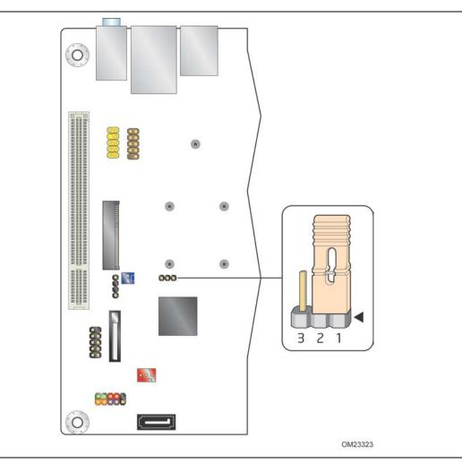
Figure 15. Location of the BIOS Configuration Jumper Block
