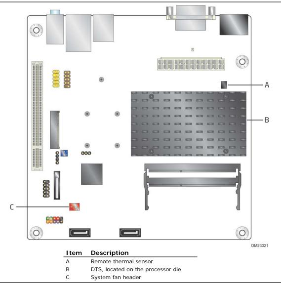
Figure 6. Thermal Sensors and Fan Header
