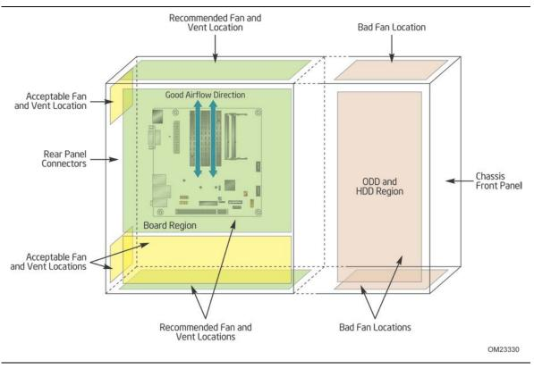
Figure 18. Fan Location Guide for Chassis Selection (Chassis Orientation is Not Restricted)
