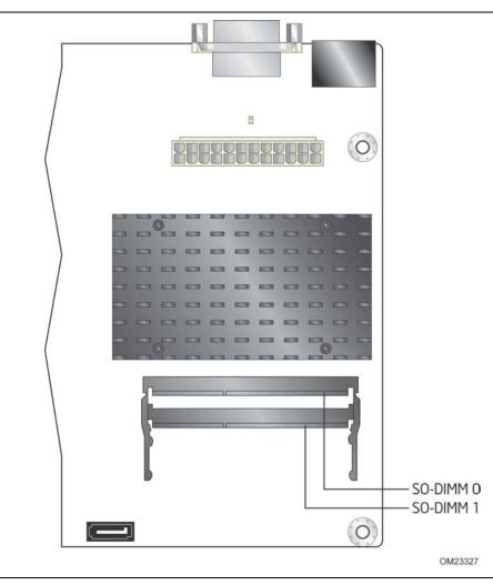
Figure 3 illustrates the memory channel and SO-DIMM configuration.
