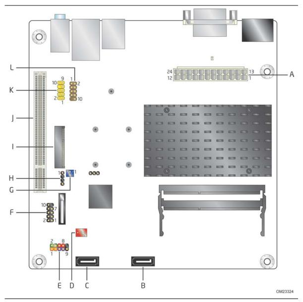
Figure 11. Component-side Connectors and Headers
