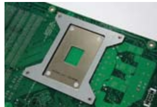
Optional heatsink bracket mounted
