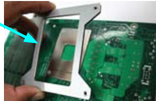
Align the Heatsink Mounting Holes (4) on the motherboard with the screw holes of the heatsink bracket
