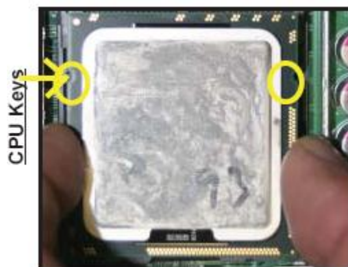
Figure 21: Aligning the CPU
