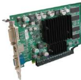
Figure 28: Install a PCI Express x16 card
