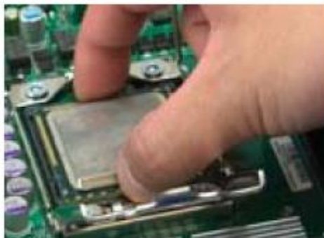
Figure 22: Ensure CPU is Properly Secured
