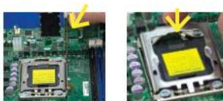
Figure 18: Lift Load Plate
