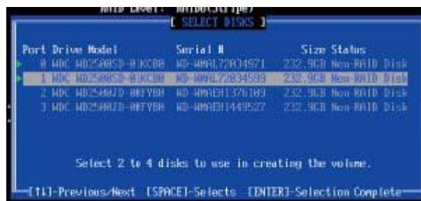
Figure 32: Selecting Drives for RAID 0 Volume
