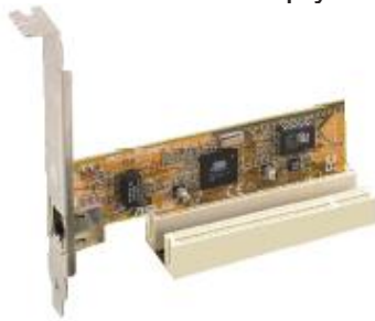
Figure 27: Installing a PCI card
