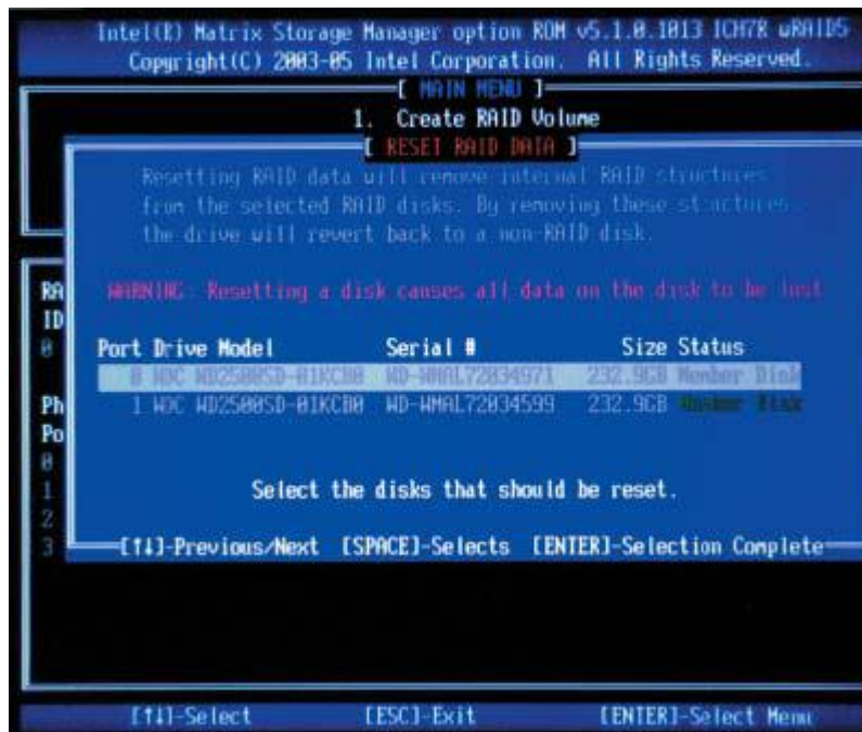
Figure 37: Resetting to Non-RAID and Resetting a RAID HDD
