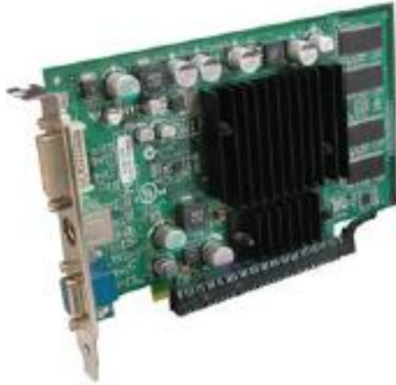
Figure 26: Install a PCI Express x16 card
