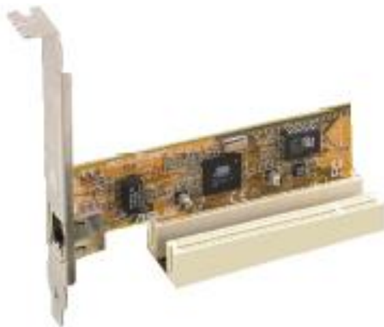
Figure 25: Installing a PCI card
