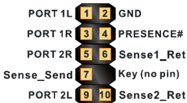
Figure 7: Front panel audio connector
