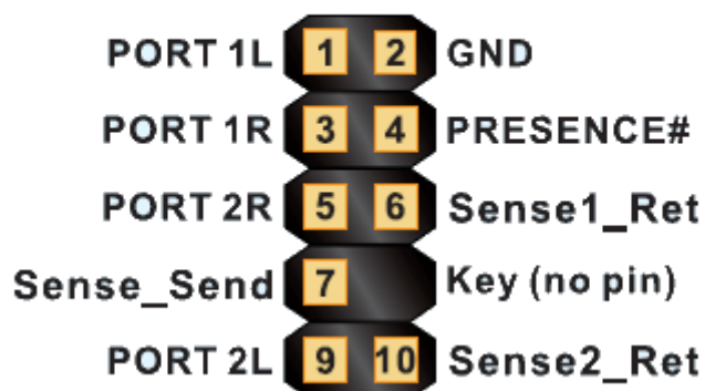
Figure 7: Front panel audio connector
