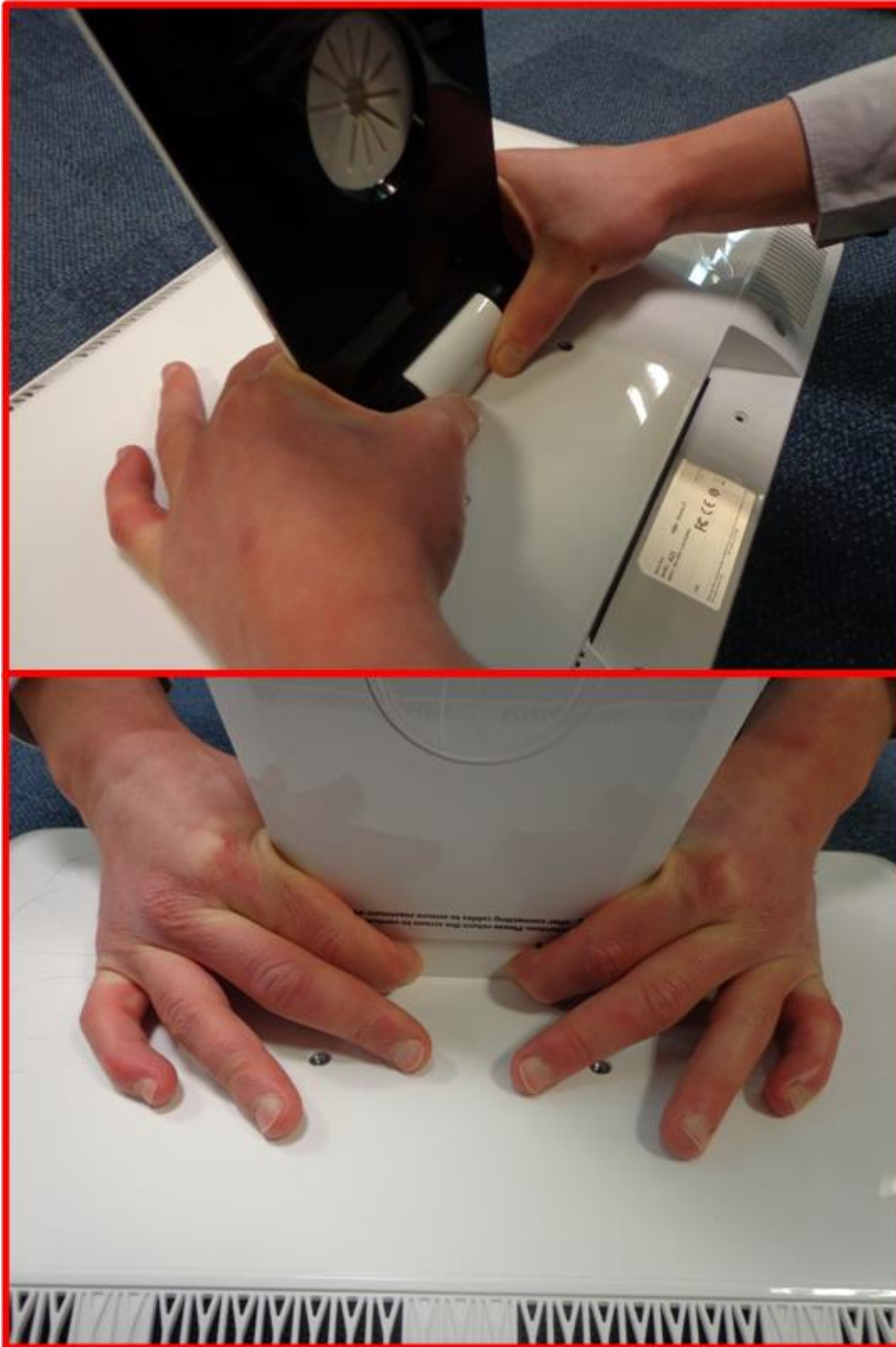
Figure 4 – Detaching the integrated chassis stand
