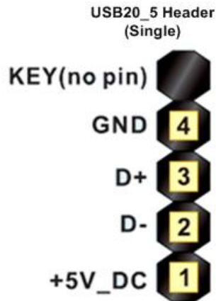
Figure 10: Front USB connector - single
