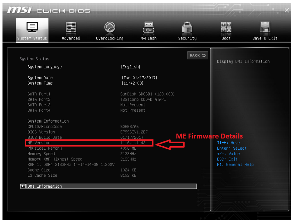
Figure 1 – BIOS screen, ME firmware information
