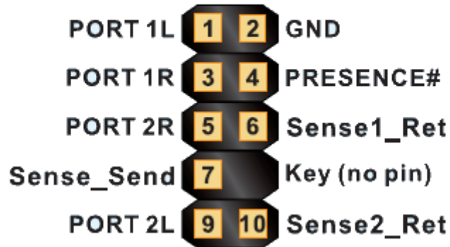
Figure 8: Front panel audio connector
