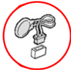
Figure 21: Removing the Battery
