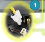
4PIN convert to 2PIN DC cable
